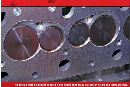
Among the more significant trends in valve engineering today are lighter weight and increased flow, with different head profiles for engines with power adders such as turbocharging, supercharging and nitrous oxide, according to one manufacturer. While keeping the valves as light as possible is essential, the challenge for engineers in optimizing valve mass is to maintain critical structural thickness so the valve can endure in these highly efficient applications, he added.
